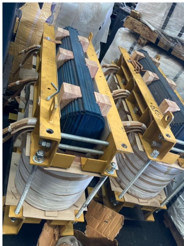
Fig 9. 650 kVA Transformer Core and Winding Assembly Under Manufacturing.
