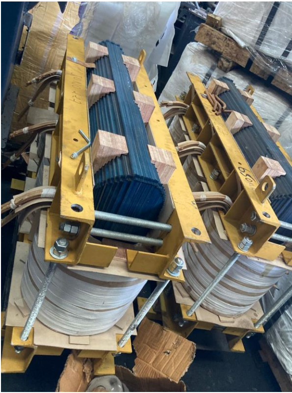
Fig 10. 650 kVA Transformer Core and Winding Assembly Under Manufacturing.
