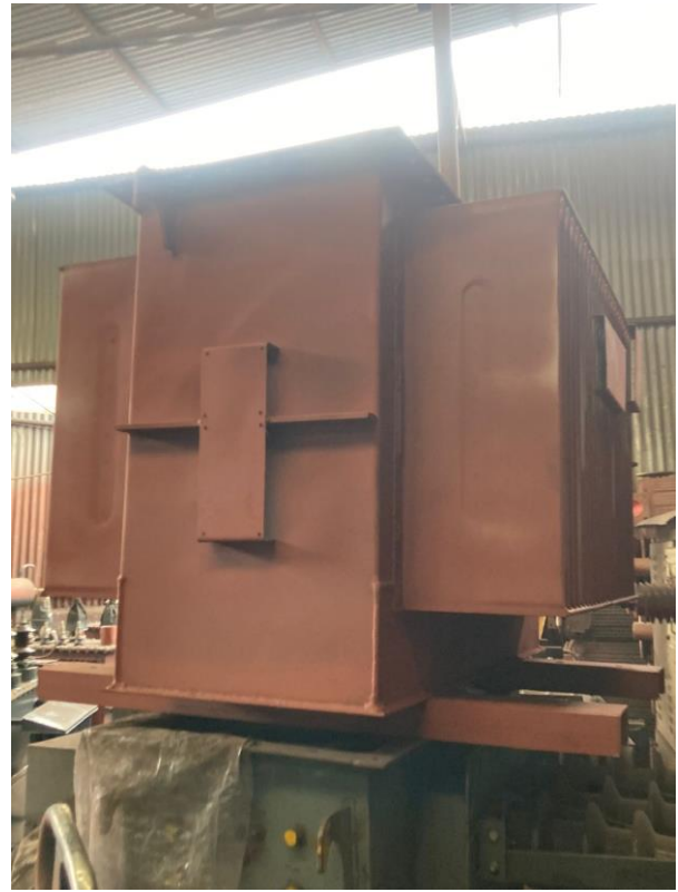
Fig 11. 650 kVA Transformer Tank Fabrication Completed.
