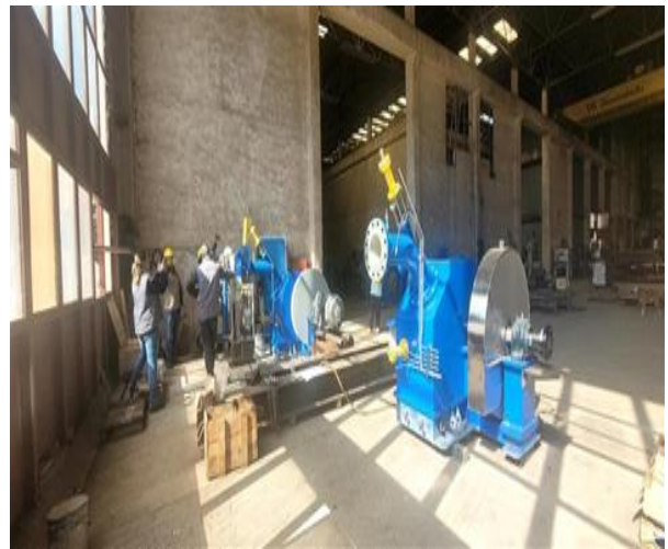
Fig.7. Turbine & assembly being prepared for testing at Factory, Greece.
