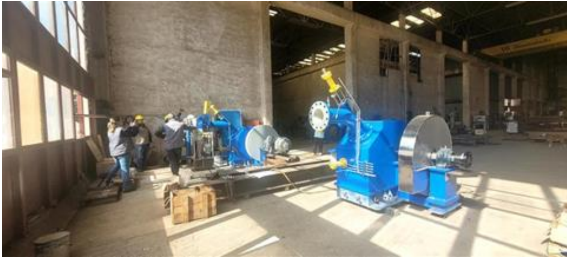
Figure 6: Turbine and assembly being prepared for testing at Factory, Greece
