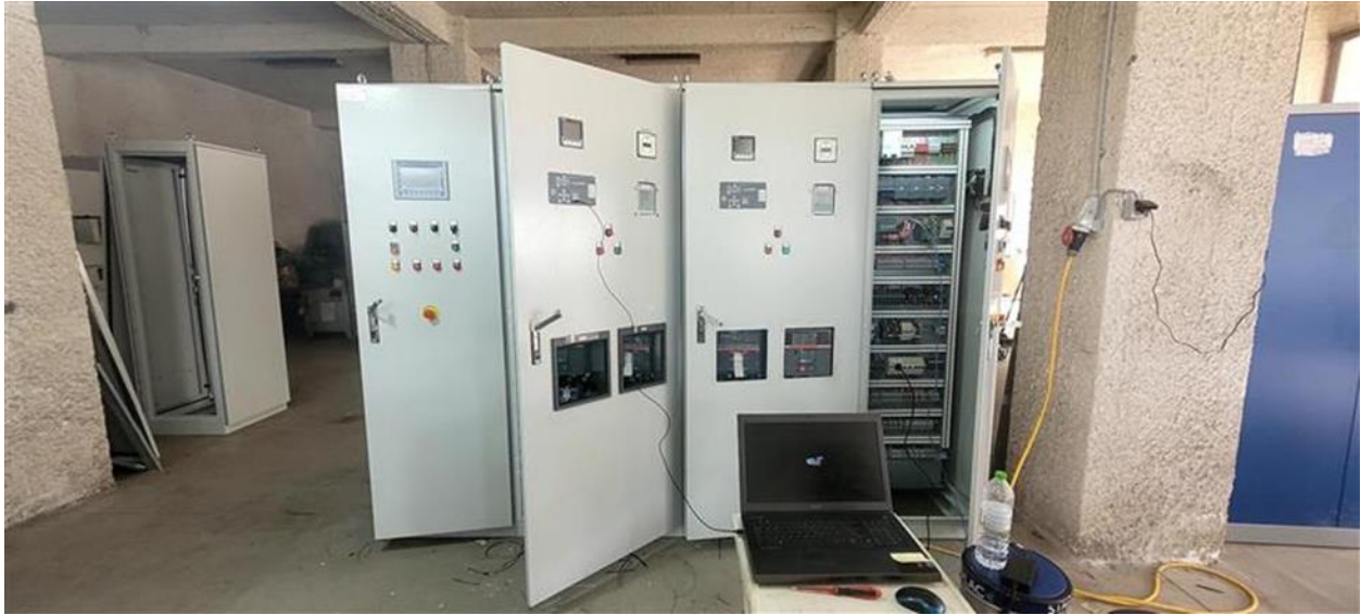
Figure 8: LV panels being tested at the factory of Poseidon FA, Greece
