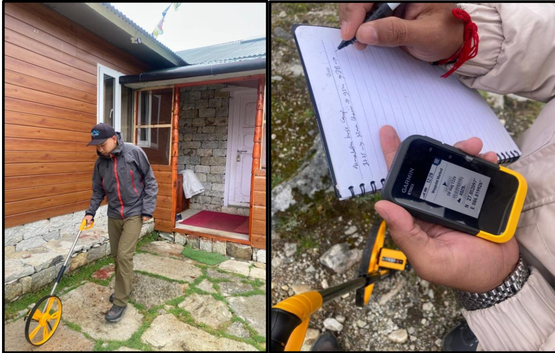
Fig.11 Service wire length measurement & DB GPS locating of Mingbo distribution plan
