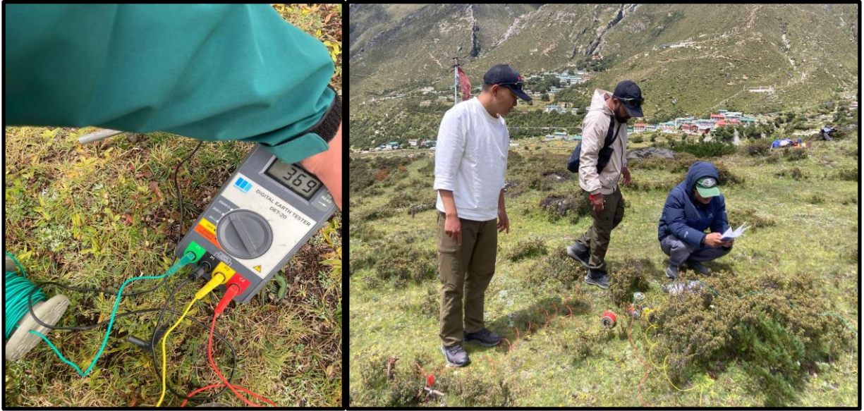
Figure 13: ERT at Power house location to test soil resistivity of Power house area
