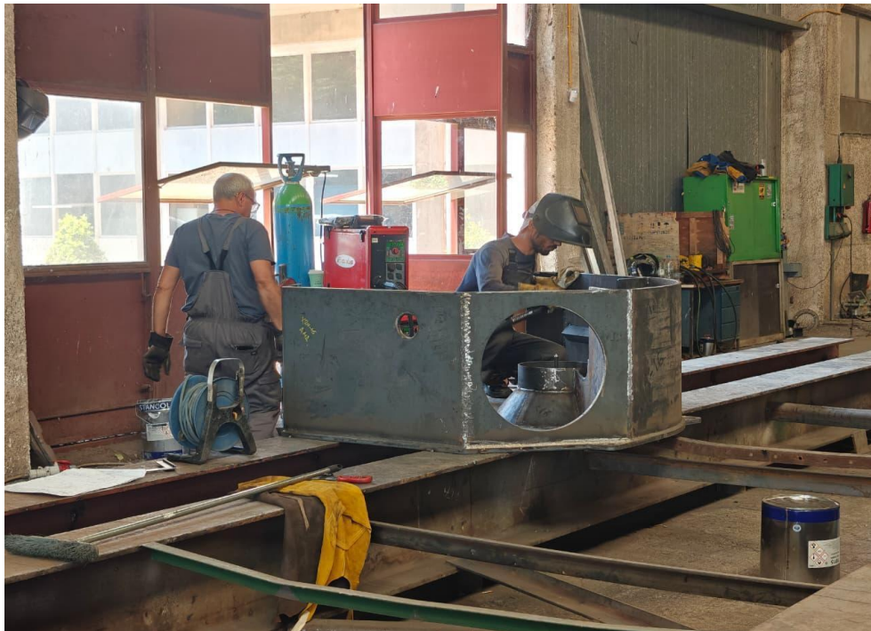
Figure 14: Fabrication of Turbine Casing, Greece
