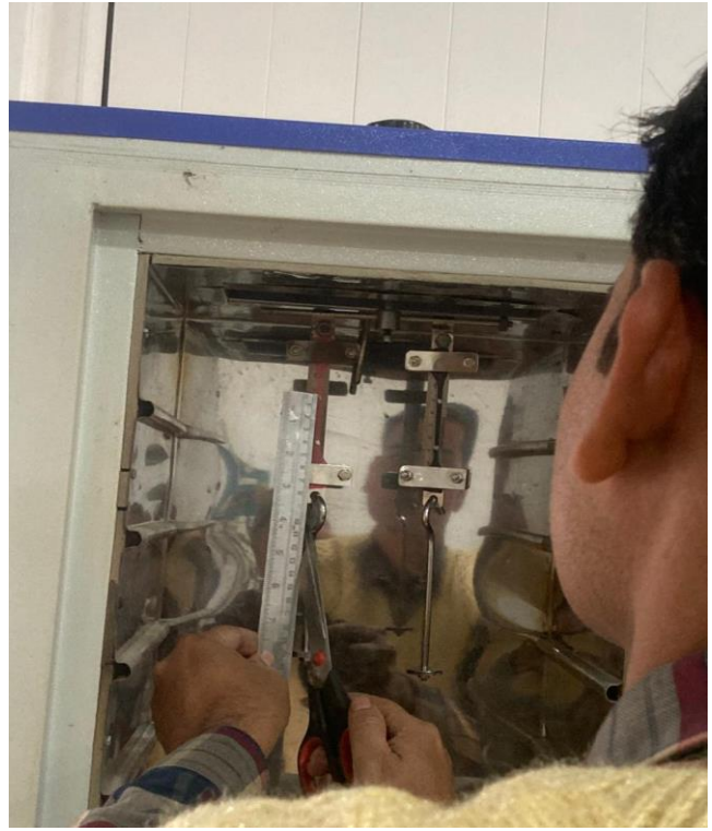
Fig4. Hot Shock Test on Cable Insulation
