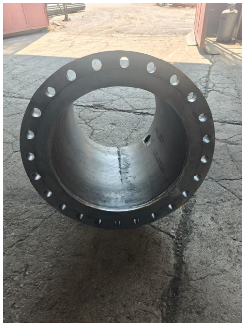
Figure 14: Fabrication of Turbine inlet, Greece
