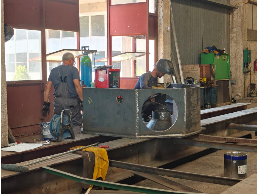
Figure 13: Fabrication of Turbine Casing, Greece
