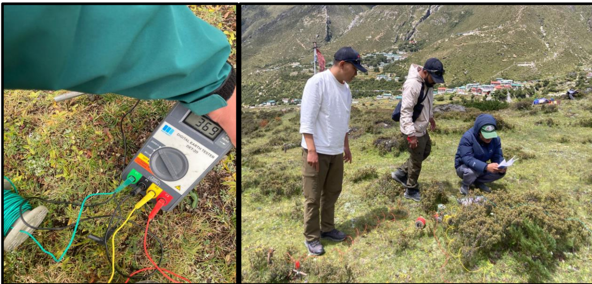
Figure 4: ERT at Power house location to test soil resistivity of Power house area
